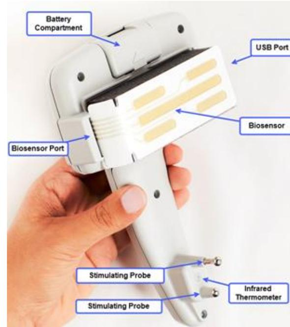
The device is powered by a 3V Panasonic CR123A battery. USB C Cable is provided for optionally uploading test results to Reporter PC application.
